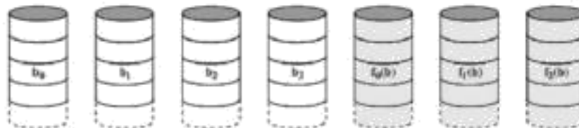
(c) RAID 2 (bit-level striping with Hamming code) Hamming kodu kadar fazla disk
